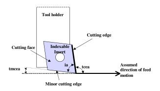
*Figure 8. Characteristics of turning tool geometry*
