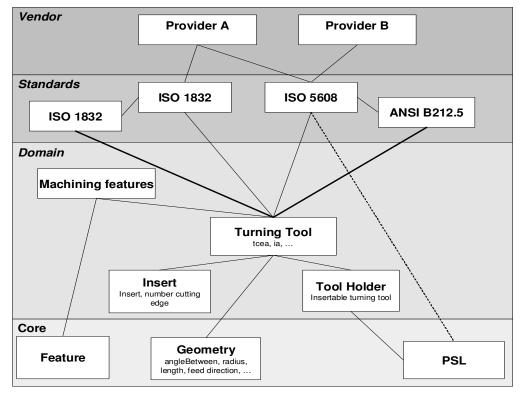
Figure 6. The four-level architecture for cutting tool ontology
