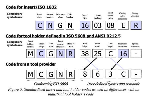
Subtle differences exist between the standardized code and the one provided by the tool provider. First, there is a difference on the dimension system, the ISO and ANSI standards use the metric, while the tool provider use the British system (inches). Therefore for a tool provider, the sixth and seventh symbols are described as: "The sixth and seventh symbol shall be a significant two-digit number that indicates the holder cross section. For shanks 5/8"
